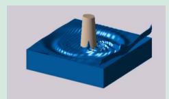
Wave forces on structure are required to design mono-piles (source TU Delft).
